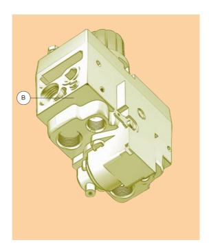
Gas flow rate adjustment to the pilot
