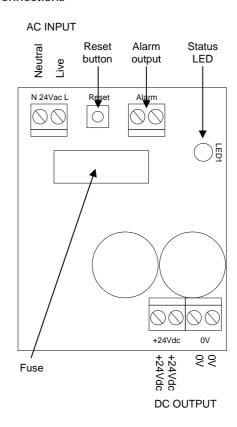
**NB** The 0V terminal on the AC input connector **is directly connected** to the 0v terminal on the DC output connector. If the DC 0V terminal is connected to equipment which will earth this connection the **0V** of the AC input will be earthed at the same time.
